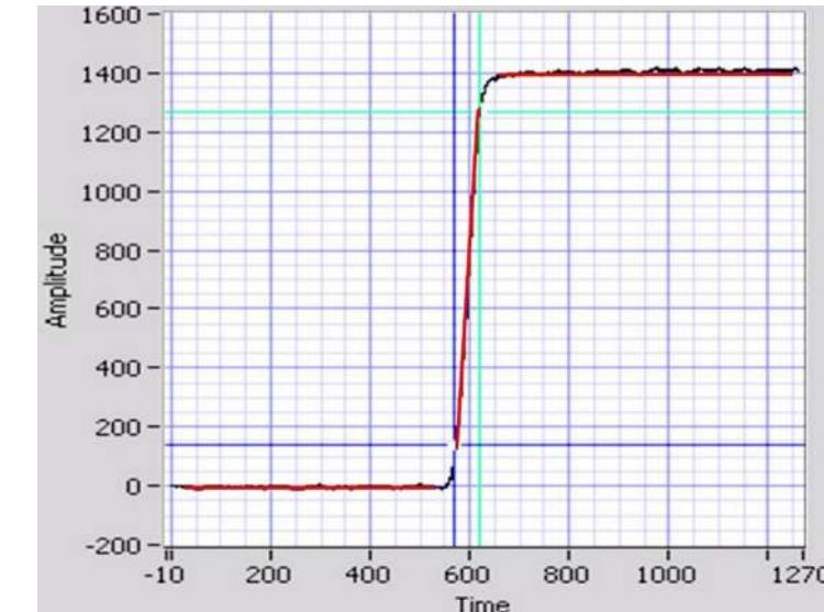
Event signal on the leakage ramp of the SDD
