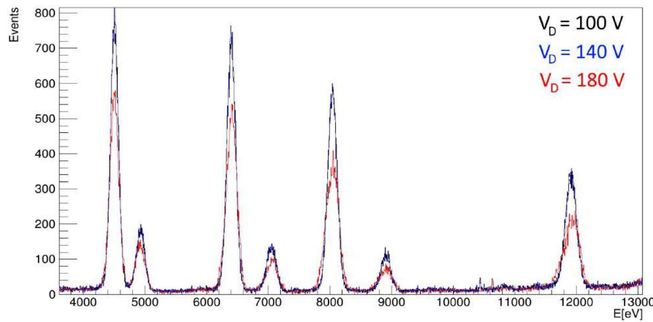
SDD linearity in function to the drift voltage
