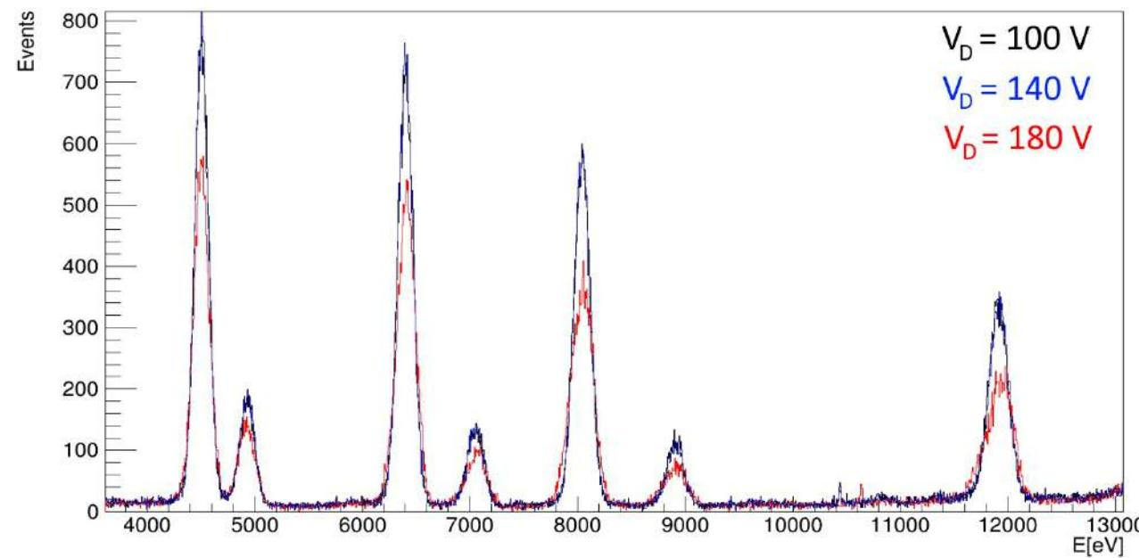
SDD gain in function to the drift voltage
