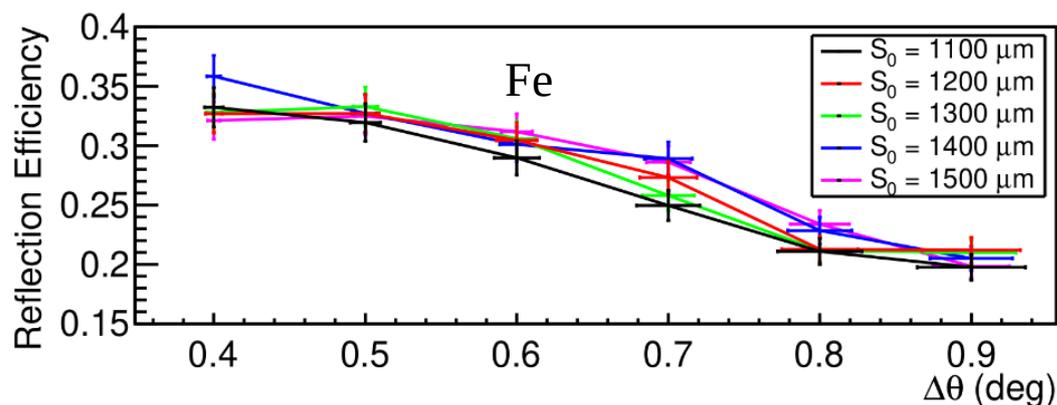
$$\epsilon_{\Delta\theta', S'_0}^R = \frac{8R_{\Delta\theta', S'_0}^B}{T_{air}R_{\Delta\theta', S'_0}^M R(S/B)A_c}$$
