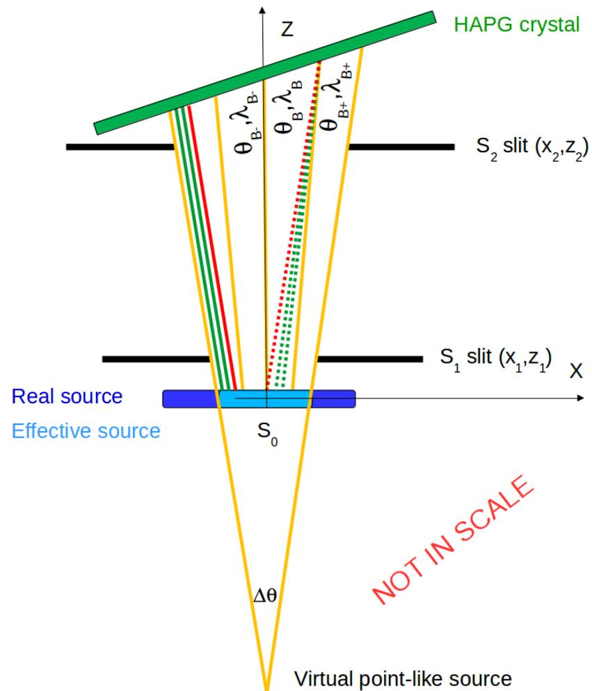
The shape of the “signal” beam can be optimized to increase the effective source size
