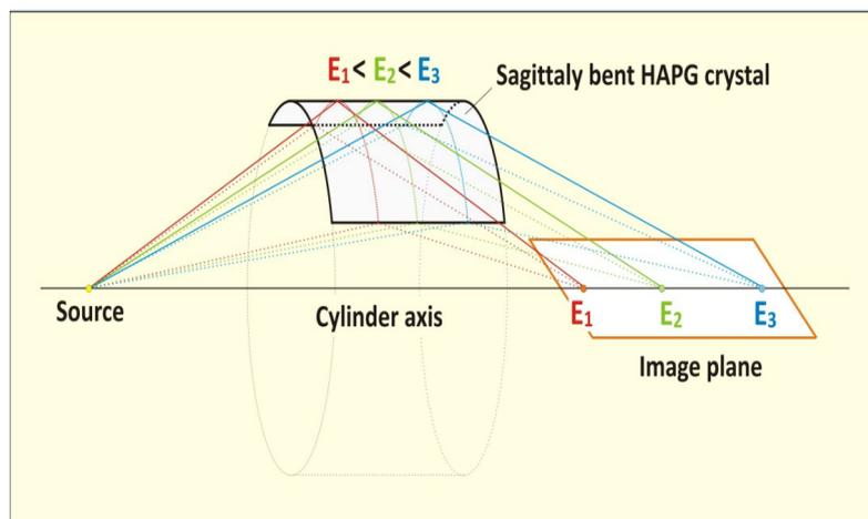
VH configuration can further improve the signal collection efficiency.
