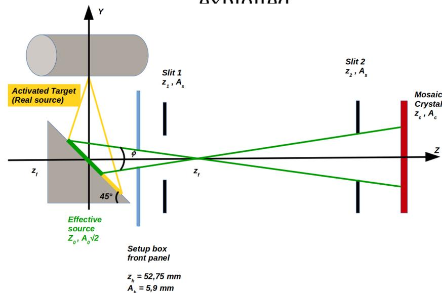
*Spectral resolution of bent HAPG/HOPG crystal is comparable to the flat one !*
