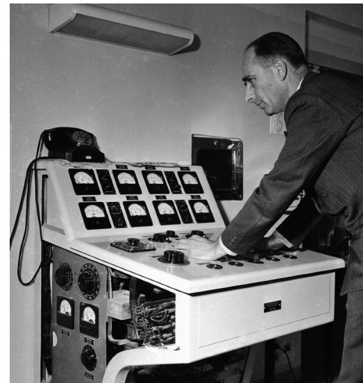
Rolf Widerøe at the control panel of a 31 MeV betatron operating since 1952 at the Norwegian Radium Hospital (Aashild)
