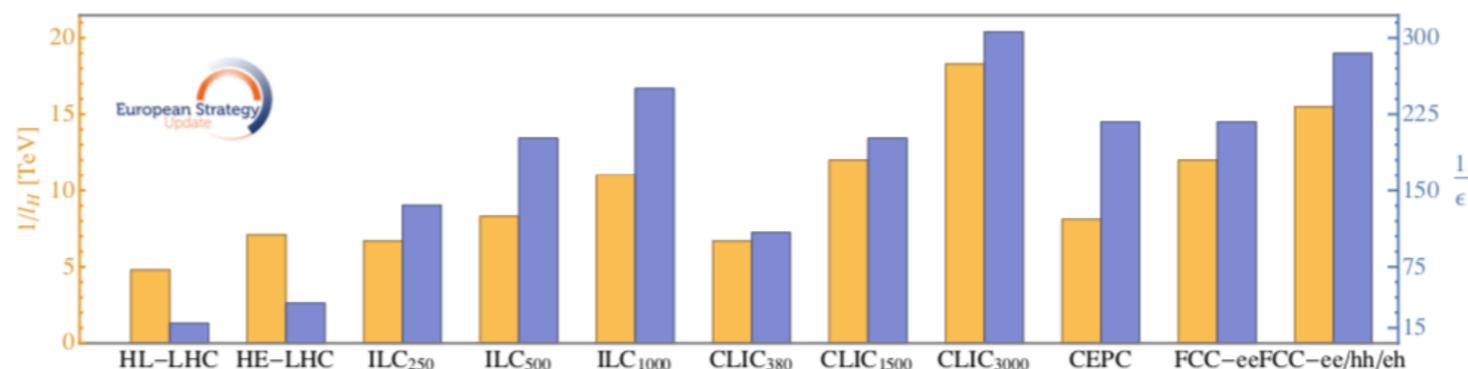
Fig. 8.5: Exclusion reach of different colliders on the inverse Higgs length  $1/\ell_H = m_*$  (orange bars, left axis) and the tuning parameter  $1/\epsilon$  (blue bars, right axis), obtained by choosing the weakest bound valid for any value of the coupling constant  $g_*$ .
