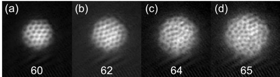
Coriolis force in rotating frame: **vortices in atomic gas**
