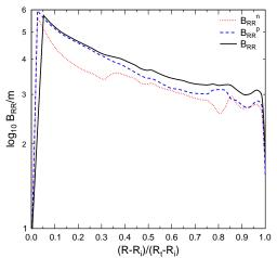
Decimal logarithm of the dimensionles RR component of nuclear inertia tensor for symmetrical fission of <sup>282</sup>Cn with linearly increasing  $R_2$ . Proton contribution is more important.
