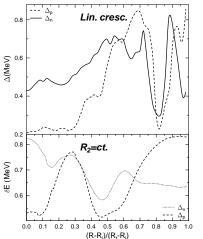
Solution of BCS equations for symmetrical fission of  $^{282}$ Cn with  $R_2$  constant (bottom) and linearly increasing (top): the gap for protons and neutrons.
