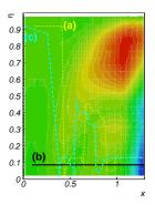
Three least action trajectories: (a) yellow dotted-line for exponentially decreasing  $R_2$ ; (b) black solid line for  $R_2$  = constant, and (c) cyan dashed-line for linearly increasing  $R_2$ .  $x = (R - R_i)/(R_t - R_i)$  and  $\eta = (A_1 - A_2)/A$  are dimensionless quantities.
