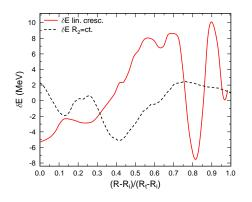
Comparison of absolute values of shell and pairing correction energies for symmetrical fission of  $^{282}$ Cn with  $R_2$  constant (dashed line) and linearly increasing  $R_2$  (solid line)
