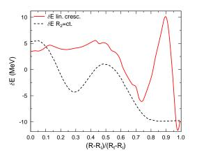
Comparison of shell plus pairing effects for fission of <sup>252</sup>Cf with linearly increasing  $R_2$  and constant  $R_2$ .
