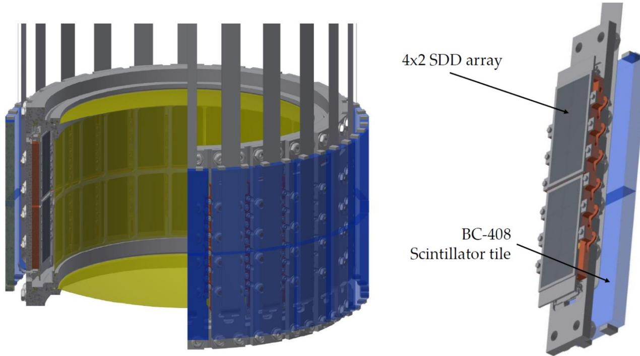
The new advance technology will allow to setup a cryogenic target detector system with an efficient detector packing density, **covering a solid angle for stopped kaons in the gaseous target of  $\sim 2\pi$ .**
