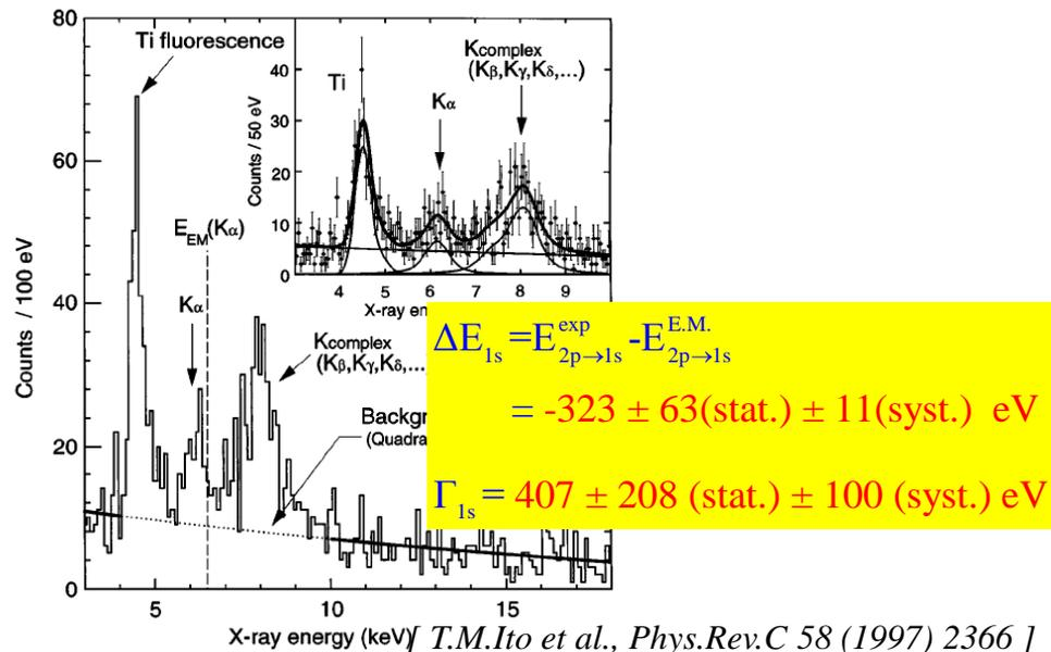
FIG. 3. Kaonic hydrogen x-ray spectrum. The inset shows the result of peak fitting and the components.
