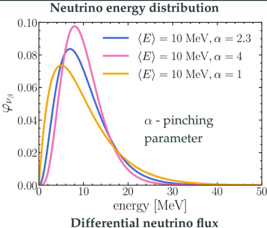
$$f_{\nu_\beta}^0(E, t_{\text{pb}}) = \frac{L_{\nu_\beta}(t_{\text{pb}})}{4\pi r^2} \frac{\varphi_{\nu_\beta}(E, t_{\text{pb}})}{\langle E_{\nu_\beta}(t_{\text{pb}}) \rangle} = \frac{F_{\nu_\beta}^0(E, t_{\text{pb}})}{4\pi r^2}$$
