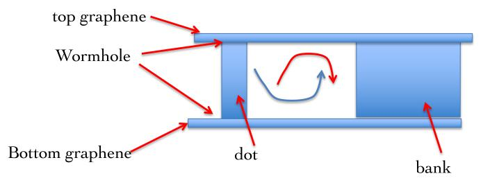
This is the pattern of a wormhole device that could be used to produce circular currents depending on the doping of graphene sheets. Advantages: **zero resistance, very small currents** (nanoampere).
