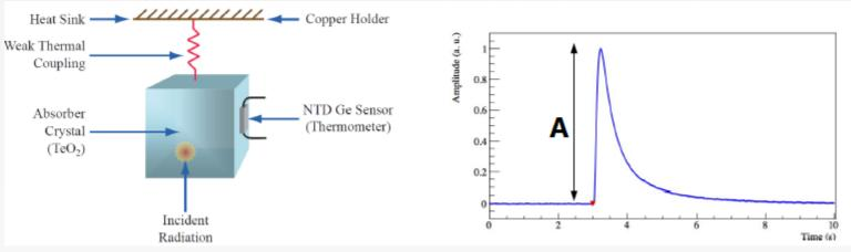
Scintillating bolometers to suppress surface contamination background
