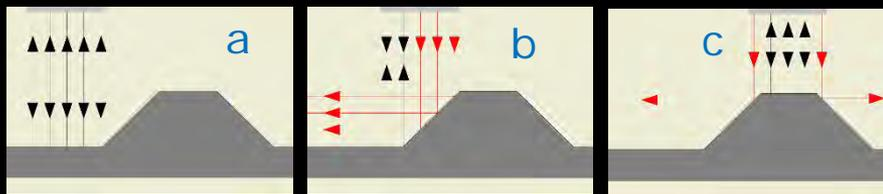
passive, radiation hard position control of the target carriage with piezo motors by measuring light reflected off a plane with grooves
