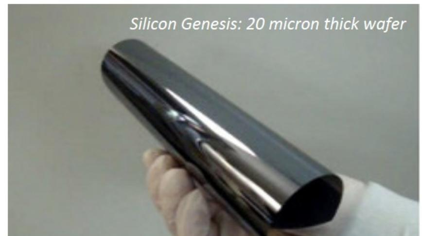
Ultra-thin chip (<50 µm): flexible with good stability
