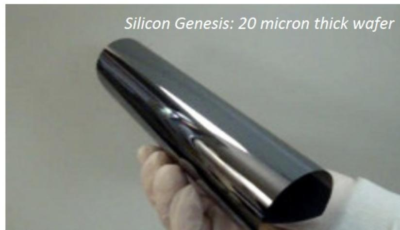
Ultra-thin chip (<50  $\mu$ m): flexible with good stability
