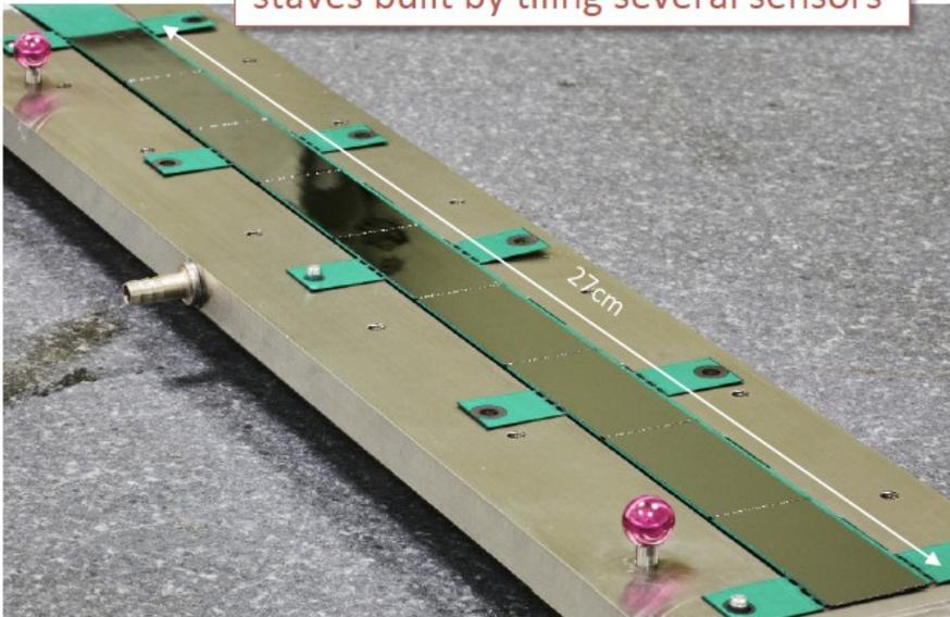
Stitching allows fabrication of sensors larger than the reticle size
