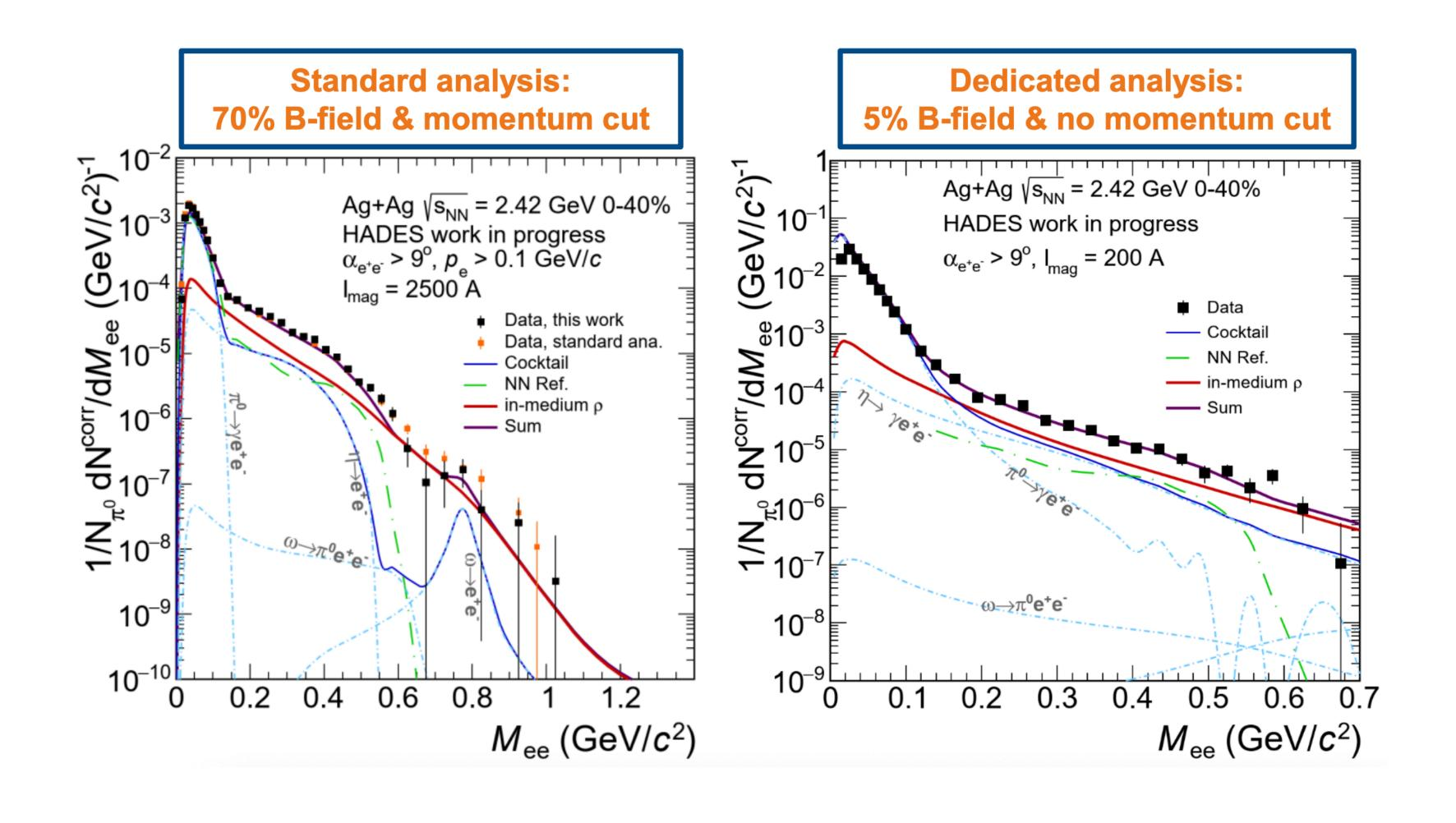
Test run with reduced field (I = 200 A)
