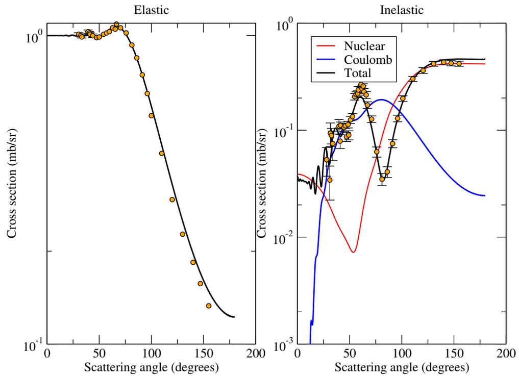
Figure 8: Left: Elastic differential cross section (relative to Rutherford cross section). Right: inelastic differential cross section.
