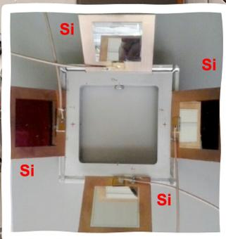
Neutron flux monitor based on  $^6\text{Li}(n,\alpha)t + \text{Si}$  detectors
