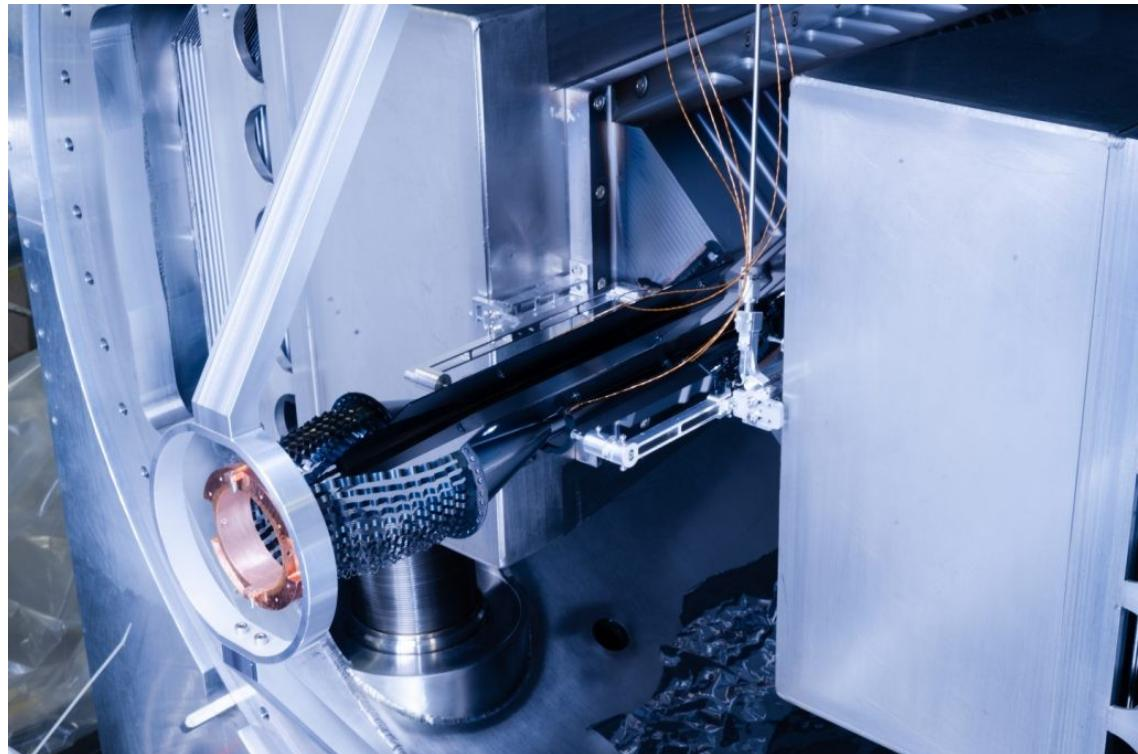
SMOG2 gas confinement cell installed in the LHCb detector,
