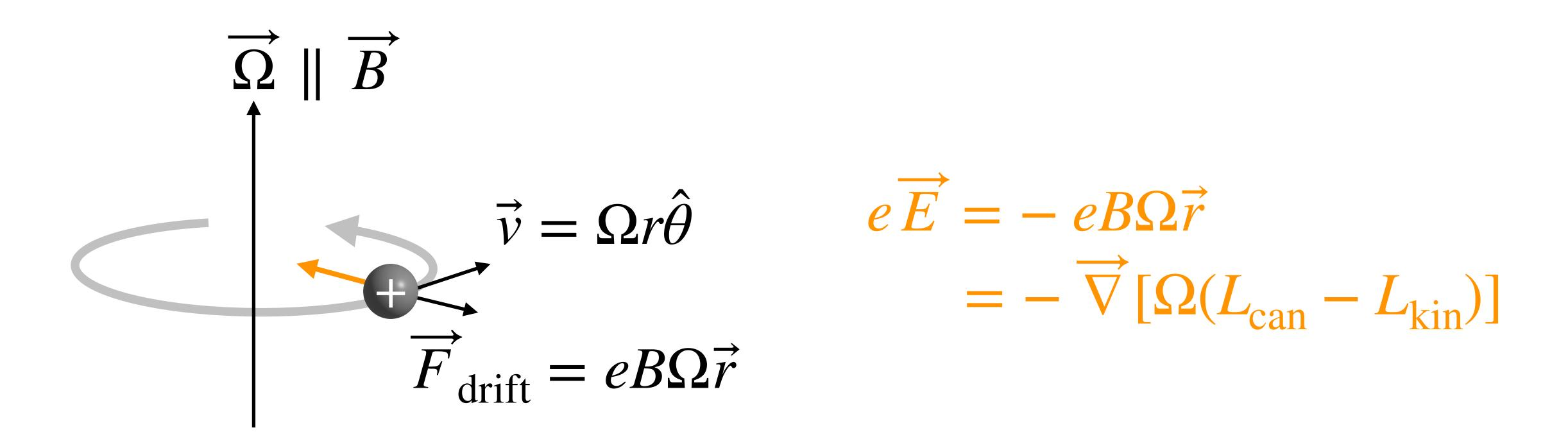
$$H + \Omega(L_{can} - L_{kin}) - \Omega L_{can} = H - \Omega L_{kin}$$
