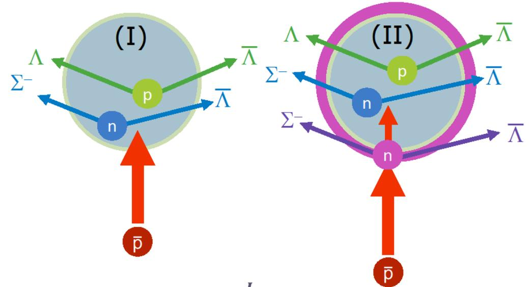
$$DR = \frac{\frac{p_{\Sigma\bar{\Lambda}}^I}{p_{\Lambda\bar{\Lambda}}^I}}{\frac{p_{\Sigma\bar{\Lambda}}^{II}}{p_{\Lambda\bar{\Lambda}}^{II}}} \sim \frac{1 + p_{abs}}{1 - p_{abs}}$$
