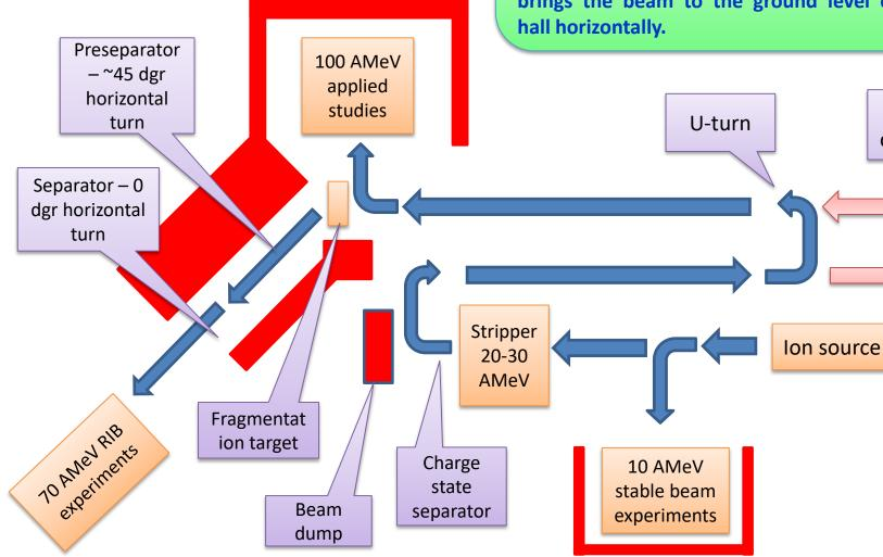
Basic considerations: LINAC-100 in trench several meters underground. U-turn for opportunity of linac main section upgrade. Beam dump for charge state separator after striper. Two experimental halls. First DFS acromat (few meters underground), horizontal total turn angle around 45 dgr. Second DFS acromat brings the beam to the ground level experimental hall horizontally.
