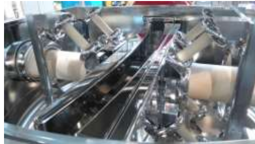
Assembled and installed the electrostatic dipoles
