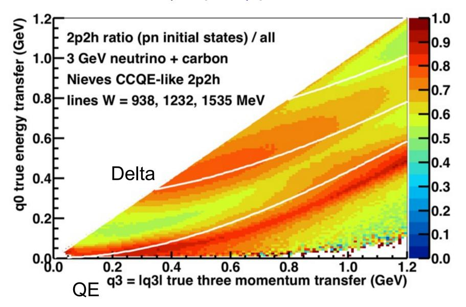
GENIE implementation uses this prediction directly by making two separate hadron tensors, one pn, one !pn, scale to other Z,A. Is not uniform, follows the interferences.
