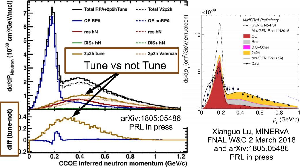
Empirical tune is adding strength to the 2p2h components in a region where three different effects may be deficient
