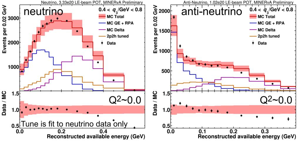
weighting up the 2p2h events with a 2D Gaussian weight this base tune designed to empirically "Fill in" the dip region not whole kinematic range. Adds ~50% overall, but x2 in dip region Improves left plot by construction, those parameters are applied to the anti-neutrino plot, which is also greatly improved!
