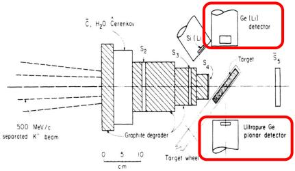
The ultrapure Ge detector is 0.4 cm thickness and has 1.8 cm of diameter, and provided a resolution of 580 eV FWHM at 85 keV
