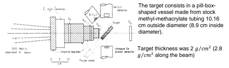
The target was filled with 99% pure isotopes of Molybdenum 92 and 98, alternatively. The flat sides of the container was of Mylar, less than 0.0127 cm thickness
