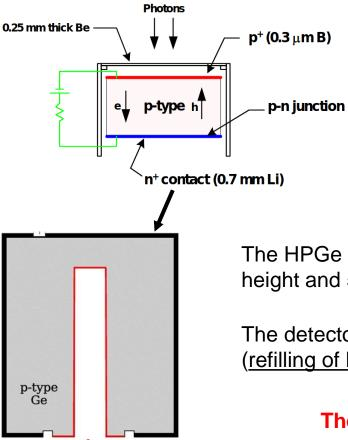
A High Purity p-type Germanium Detector (HPGe), designed by Baltic Scientific 253 Instruments, could be used covering a wide energy range from hundred keV to a few MeV.
