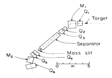
Kaons and other particles produced in the forward diections entered a mass spectrometer, consisting of 6 Quadrupoles (Q) two bending magnets (M), a separator and a «mass» slit.
