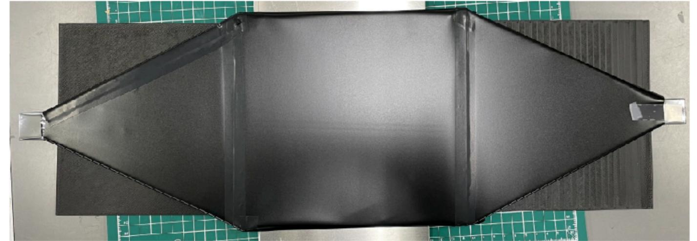
Kaon detector wrapped with aluminized mylar
