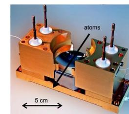
High-Q superconducting Microwave cavity
