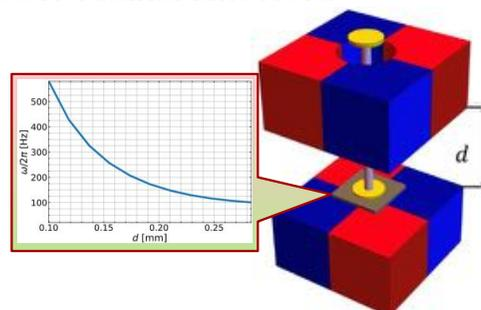
Use magnetically levitated cavity optomechanics to measure displacement to a resolution of
