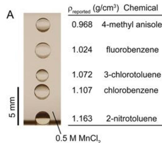
"Axial" Magnetic Levitation Using Ring Magnets Enables Simple Density-Based Analysis, Separation, and Manipulation
