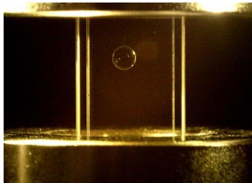
Measure droplet height as we vary the magnet separation and compare with theory –
