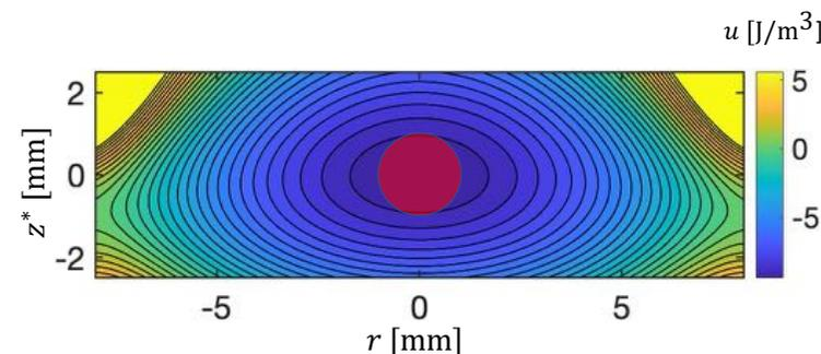
Potential Energy of the trap – Red Ball is the droplet – for intermagnet separation of 7 mm
