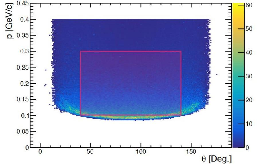
FIG. 15: Simulated deuteron acceptance in ALERT as a function of momentum and scattering angle. The colors indicate the total energy deposition of the
