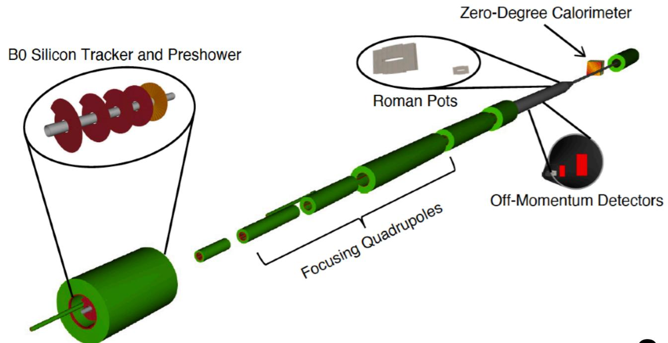
Magnetic spectrometer and detectors for charged particles, integrated in accelerator optics, several subsystems
