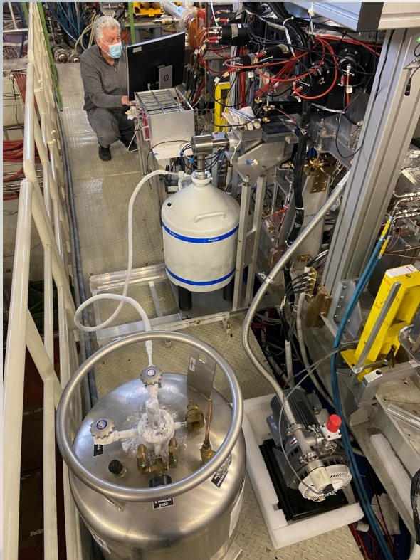
Ge refilling procedure to be done each 7-10 days
