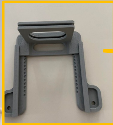
Pb target support behind luminometer
