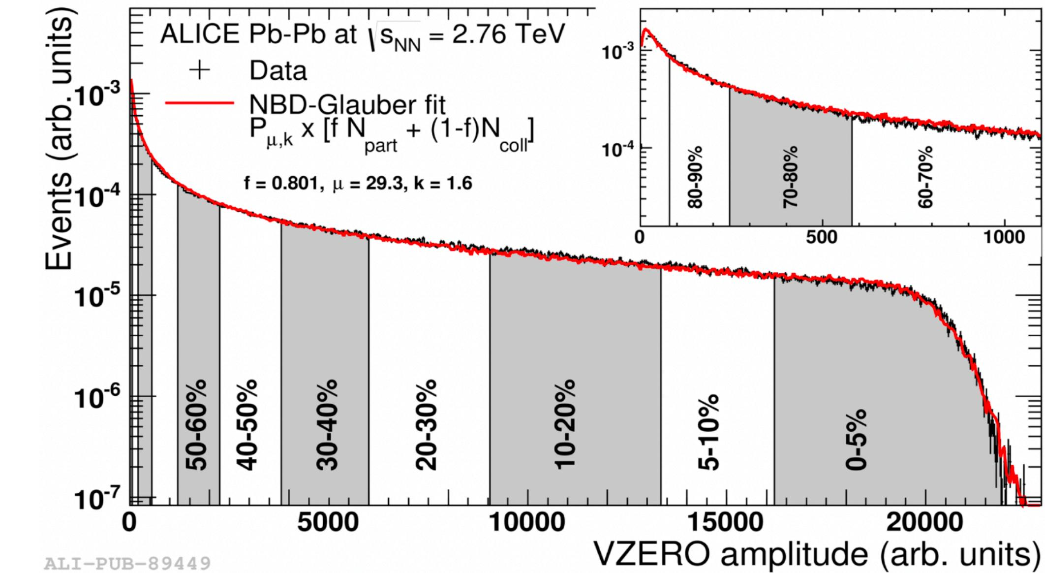
Centrality classes defined experimentally by integrating the amplitude distribution measured by the V0 scintillators
