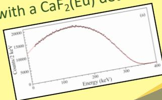
Observation of correlated  $e^+e^-$  pairs emission in  $\alpha$  decay of  $^{241}\text{Am}$  ( $A_{e^+e^-}/A_\alpha \approx 5 \times 10^{-9}$ )
