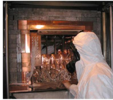
As a result of a 2nd generation R&D for more radiopure NaI(Tl) by exploiting new chemical/physical radiopurification techniques (all operations involving - including photos - in HP Nitrogen atmosphere)
