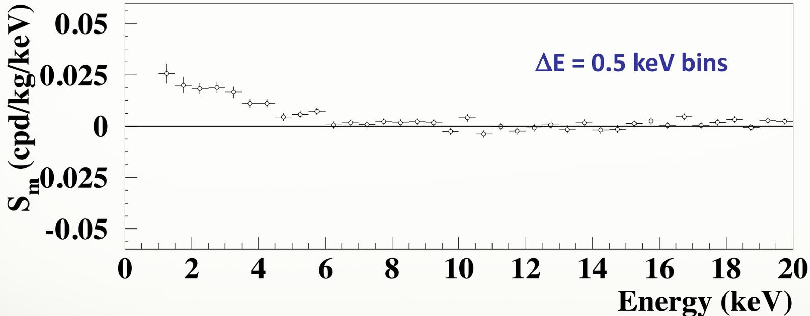
A clear modulation is present in the (1-6) keV energy interval, while  $S_m$  values compatible with zero are present just above
