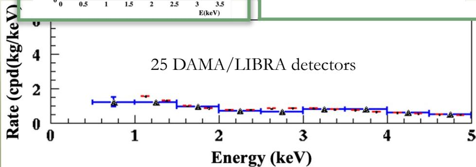
Energy spectrum of the *single-hit* scintillation events – already corrected for the efficiencies – in the new configuration (blue, exposure 2350 kg×d) and in DAMA/LIBRA–phase2 (red, the energy threshold was 1 keV, 1.53 ton×yr).
