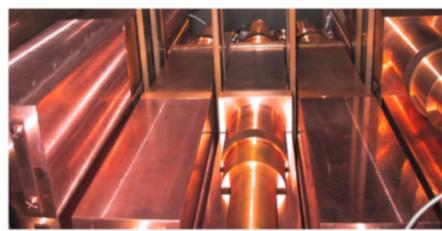
Residual contaminations in the new DAMA/LIBRA NaI(Tl) detectors:  $^{232}\text{Th}$ ,  $^{238}\text{U}$  and  $^{40}\text{K}$  at level of  $10^{-12}$  g/g
