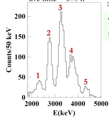
$^{238}\text{U}$  chain splitted into 5 subchains:  $^{238}\text{U} \rightarrow ^{234}\text{U} \rightarrow ^{230}\text{Th} \rightarrow ^{226}\text{Ra} \rightarrow ^{210}\text{Pb} \rightarrow ^{206}\text{Pb}$
