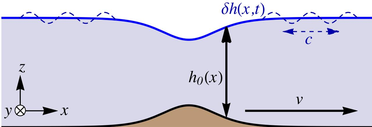
$$\text{Flow velocity } v = \frac{q}{h}$$
