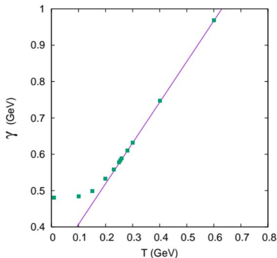
The line is the fit  $\gamma = \gamma_0 + bT$  with  $\gamma_0 = 0.295$  GeV and  $b = 1.12$ .
